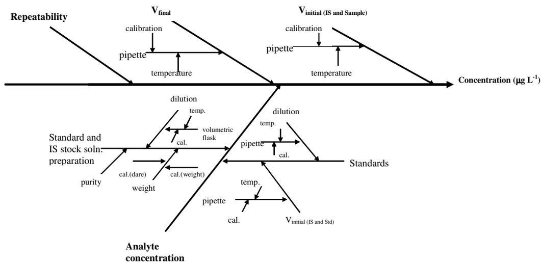
**Figure 1.** Cause and effect diagram for the determination of 25-OH vitamin D<sub>3</sub> and D<sub>2</sub>
