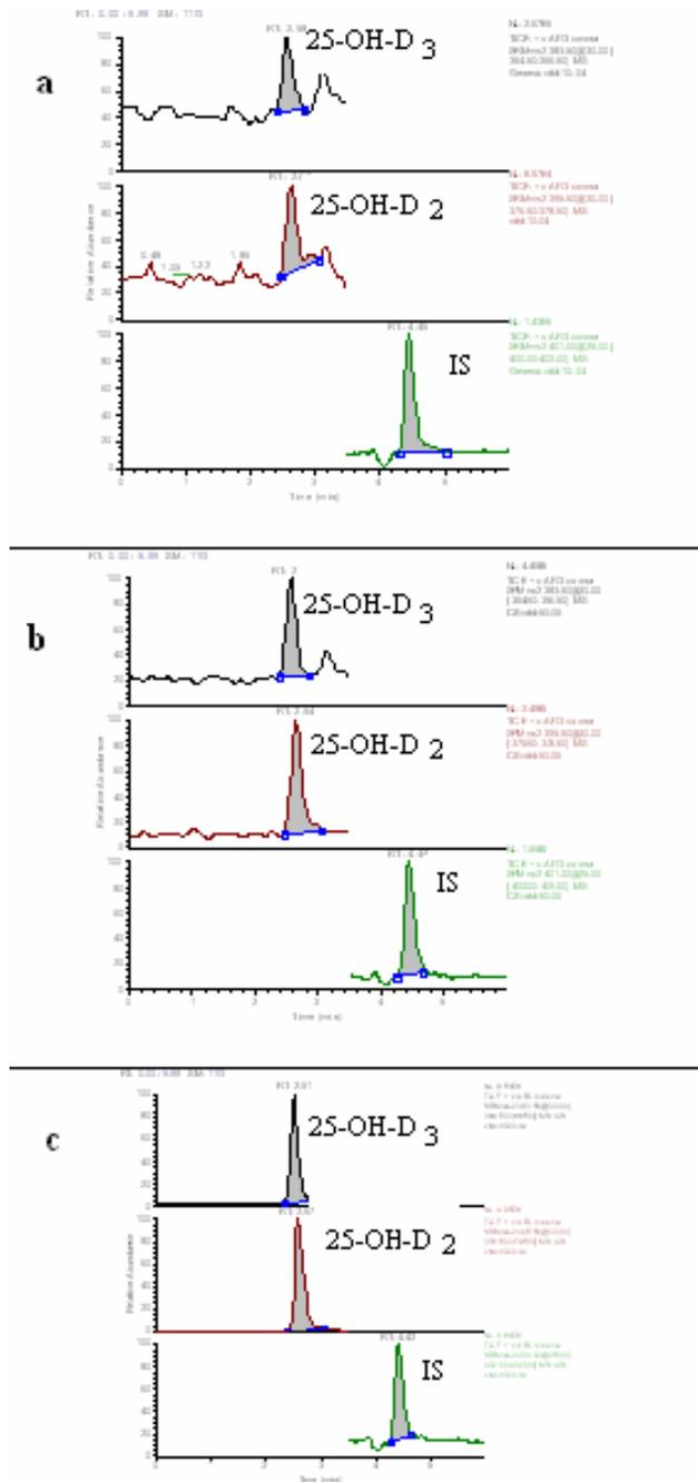
**Figure 2.** Sample chromatograms of 25-OH Vitamin D<sub>3</sub> and D<sub>2</sub> from spiked serum with ion trap LC/MS/MS a) 50 µg L<sup>-1</sup> b) 100 µg L<sup>-1</sup> c) 100 µg L<sup>-1</sup>
