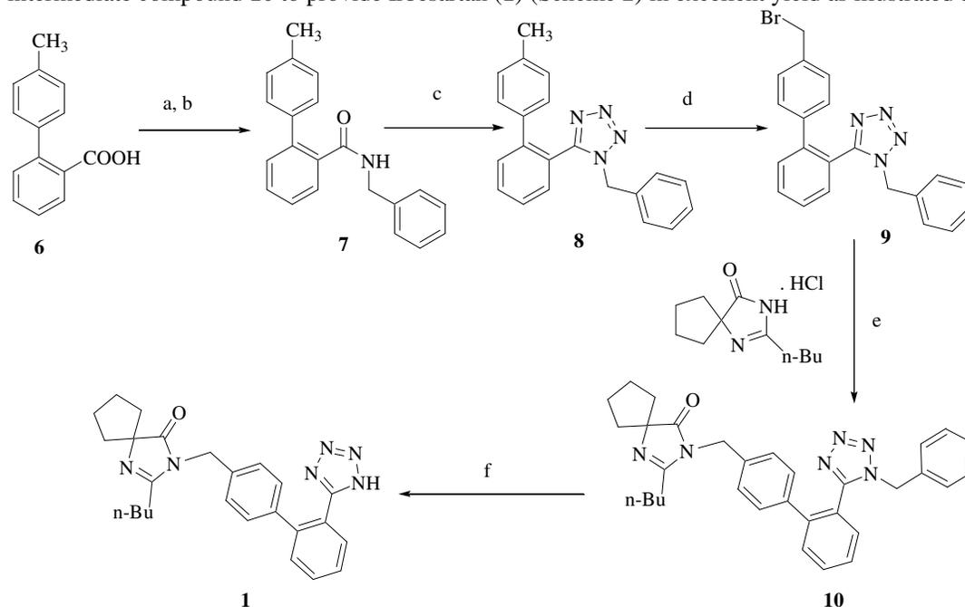
**Scheme 2.** Reagents and conditions: (a) SOCl<sub>2</sub>, TEA, toluene, 20-25°C, 2 h. (b) benzylamine, 20-25°C, 4h, 95% for two steps. (c) triphenylphosphine / diethyl azodicarboxylate (DEAD) / trimethylsilylcyaniide, THF, 20-25°C, 24 h, 91%. (d) DBDMH, AIBN, EtOAc, reflux, 6 h, 89%. (e)
