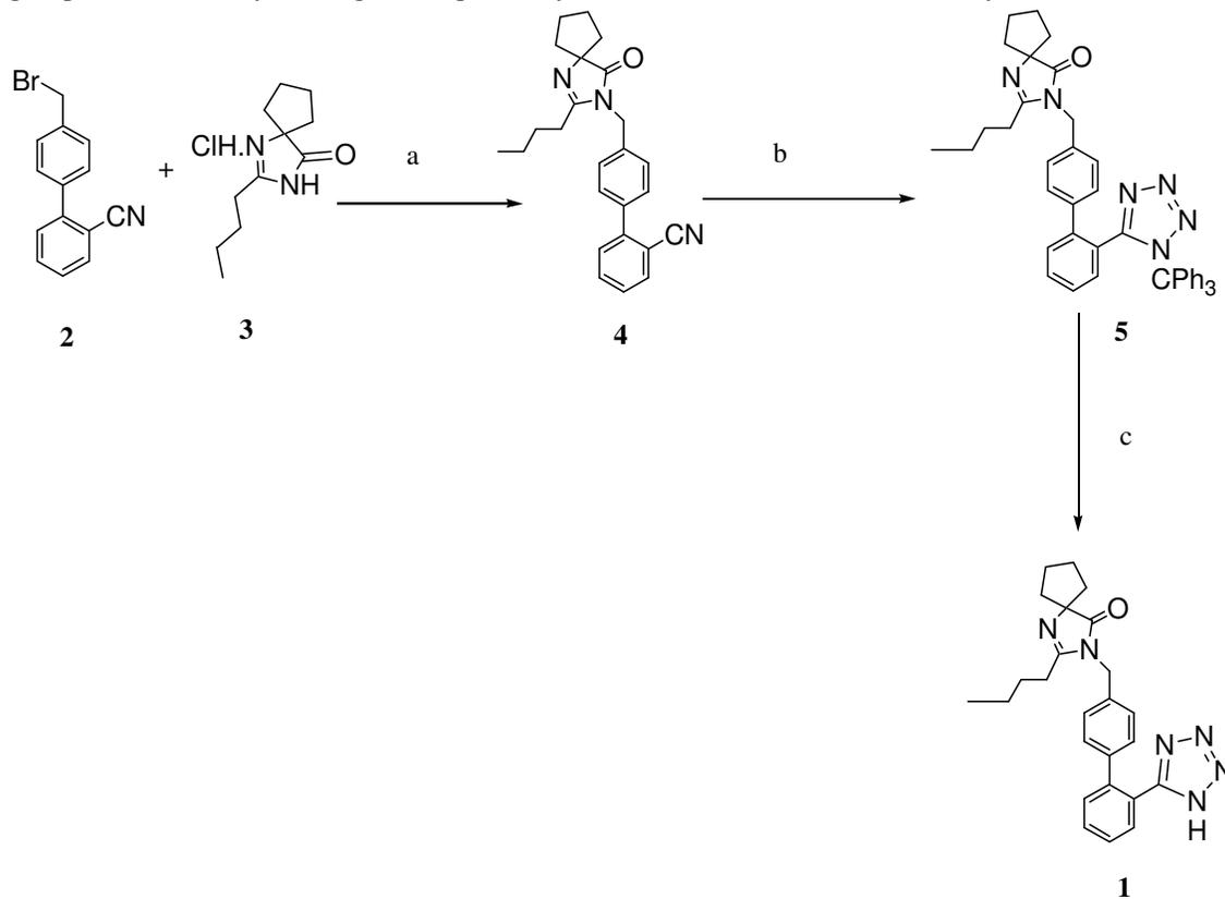
**Scheme 1.** Reagents and conditions: (a) NaH, DMF, rt, 1 h, 79%. (b) tributyltin azide, xylene, reflux, 66 h, trityl chloride, 26 h, 72%. (c) 4N HCl, methanol, THF, rt, 4 h, 67%.
