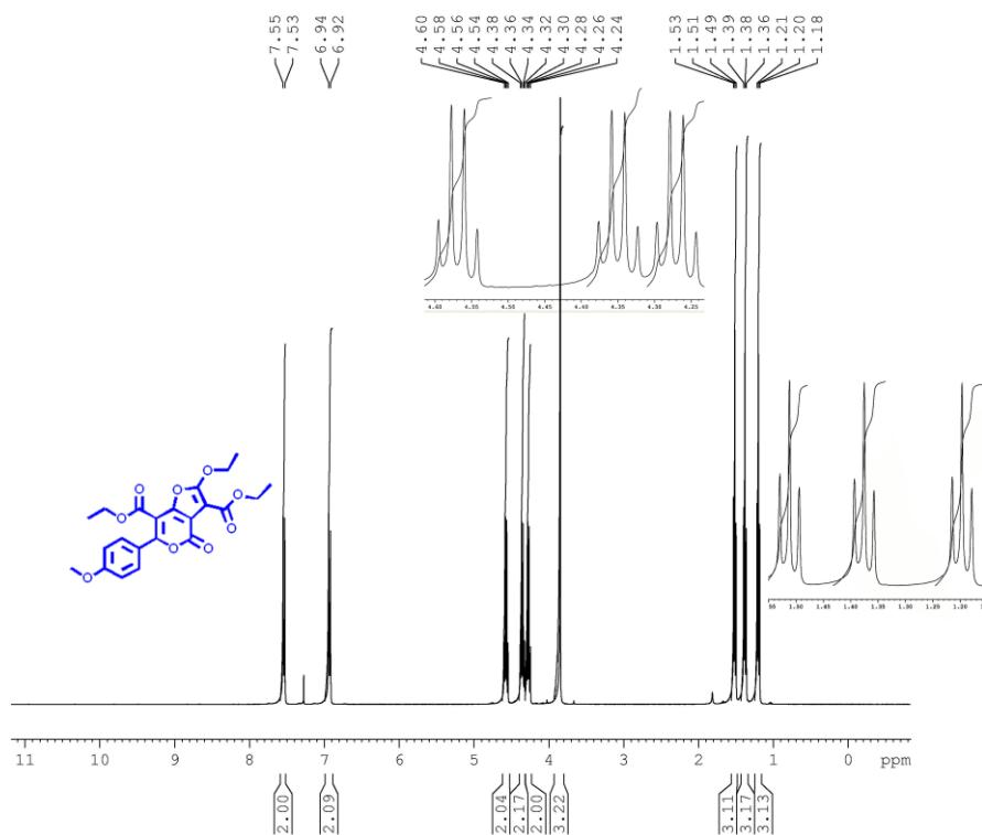
**Figure 3.**  $^1\text{H}$  NMR spectra of compound **3a**
