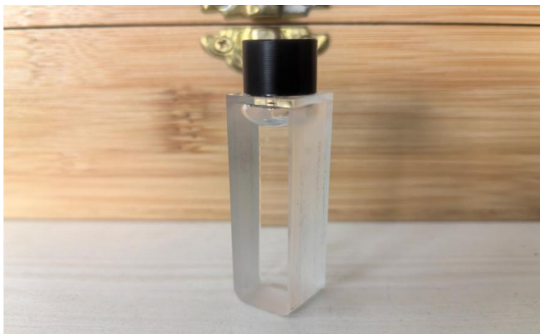
Figure 3. Sealed short-wavelength near-infrared wavelength standard solution material
