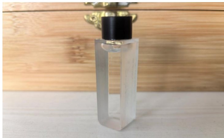
Figure 3. Sealed short-wavelength near-infrared wavelength standard solution material
