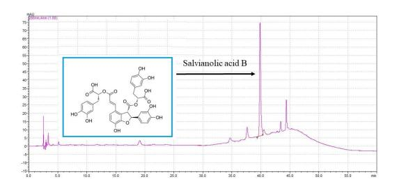
Figure S1: Chemical structure, and HPLC chromatogram of salvianolic acid B
